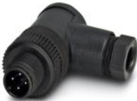
Sensor/actuator connector, male, angled, 4-pos., M12, A-coded, screw connection, plastic knurl, cable screw connection Pg7
