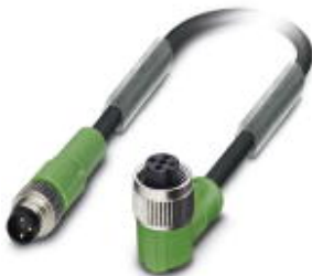
Sensor/Actuator cable, 3-position, PUR halogen-free, Black-gray RAL 7021, Plug straight M8, on Socket angled M12, A-coded, Cable length: 3 m
