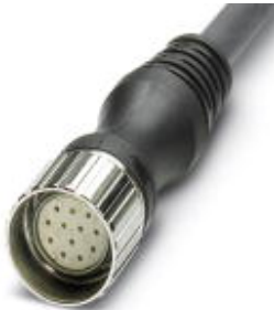
M23 socket, straight, 12-pos., with 10 m master cable, pin 9 and 10 bridged
