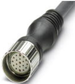
Female connector, Number of positions: 19, Status indication: No; Master cable connection: M23 socket, Cable length: 5 m, Shielding: No
