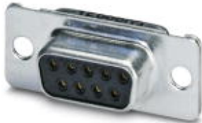
D-SUB contact insert, shell size 1, with nine signal contacts, contact type socket, with solder cup, straight, fixing with a 3 mm hole, for panel mounting frame and sleeve housing VS-09-...
