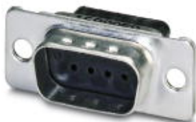
D-SUB contact carrier, shell size 1, for nine signal contacts, contact type pin, for crimp contacts, straight, fixing with 3 mm hole, for panel mounting frame and sleeve housing VS-09-...
