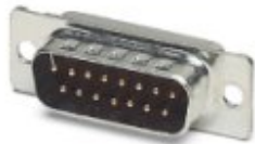
D-SUB contact insert, shell size 2, with 15 signal contacts, contact type pin, with solder cup, straight, fixing with a 3 mm hole, for panel mounting frame and sleeve housing VS-15-...
