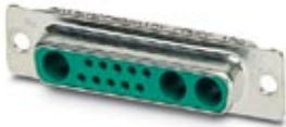
D-SUB contact insert, shell size 3, with ten signal contacts with solder cup, straight, accommodation for three combined contacts, contact type socket, fixing with a 3 mm hole, for panel mounting frame and sleeve housing VS-25-...
