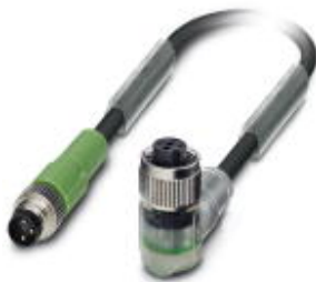
Sensor/Actuator cable, 3-position, PUR halogen-free, Black-gray RAL 7021, Plug straight M8, on Socket angled M12, A-coded, with 2 LEDs, Cable length: 3 m
