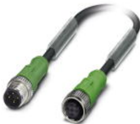
Sensor/Actuator cable, 4-position, PUR halogen-free, Black-gray RAL 7021, Plug straight M12, A-coded, on Socket straight M12, A-coded, Cable length: 2 m
