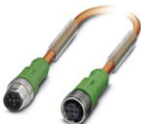
Sensor/Actuator cable, 5-position, PUR halogen-free, Irradiated, orange RAL 2003, Plug straight M12, A-coded, on Socket straight M12, A-coded, Cable length: 0.6 m, Customer version
