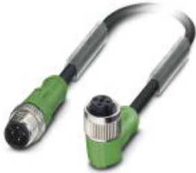
Sensor/Actuator cable, 4-position, PUR halogen-free, Black-gray RAL 7021, Plug straight M12, A-coded, on Socket angled M12, A-coded, Cable length: 5 m
