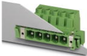
Plug component, Nominal current: 76 A, Rated voltage (III/2): 1000 V, Number of positions: 3, Pitch: 10.16 mm, Connection method: Screw connection, Color: green, Contact surface: Silver
