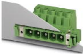
Plug component, Nominal current: 76 A, Rated voltage (III/2): 1000 V, Number of positions: 5, Pitch: 10.16 mm, Connection method: Screw connection, Color: green, Contact surface: Silver
