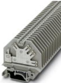
Feed-through terminal block, Connection type: Screw connection, Slip-on connection, Cross section: 0.2 mm 2 - 4 mm 2 , AWG :24- 14, Width: 6.2 mm, Color: gray, Mounting: NS 32
