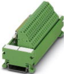
VARIOFACE module, with spring-cage connection and D-Subminiature socket strip, for mounting on NS 35/7.5, 15-pos.
