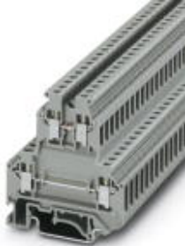
Feed-through terminal block, Cross section: 0.2 mm 2 - 4 mm 2 , AWG: 24 - 12, Connection type: Screw connection, Width: 6.2 mm, Color: blue, Mounting type: NS 35/7,5, NS 35/15, NS 32
