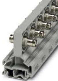
BNC connector, single-level, for mounting on NS 32 or NS 35/7.5, wave impedance: 75 Ohm
