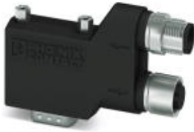
D-SUB plug, 9-pos., pin, assignment: 3, 5, 6, 8; two M12 cable glands (B-coded) under 90°. Bus system: PROFIBUS DP up to 12 Mbps. Termination resistor via separate M12 terminator.
