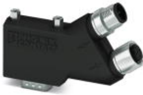
D-SUB plug, 9-pos., pin, assignment: 3, 5, 6, 8; two M12 cable glands (B-coded) under 35°. Bus system: PROFIBUS DP up to 12 Mbps. Termination resistor via separate M12 terminator.
