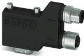
D-SUB plug, 9-pos., socket, assignment: 2, 3, 5, 6, 7, 9; two M12 cable glands (A-coded) under 90°. Bus system: CAN, CANopen®. Termination resistor via separate M12 terminator.
