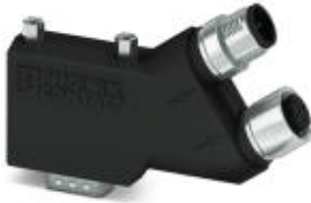
D-SUB plug, 9-pos., socket, assignment: 2, 3, 5, 6, 7, 9; two M12 cable glands (A-coded) under 35°. Bus system: CAN, CANopen®. Termination resistor via separate M12 terminator.
