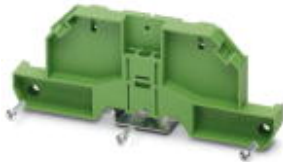
Lateral element, to attach profile cover UM 122 to DIN rail NS 35/7.5, with M3 screw fixture, tightening torque 0.5 Nm ... 0.6 Nm
