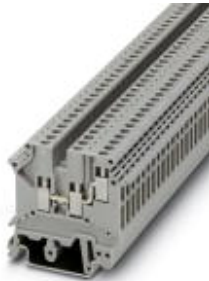
1-level terminal block with double connection on one side, cross section: 0.2 - 2.5 mm 2 , AWG: 30 - 12, width: 5.2 mm, color: gray
