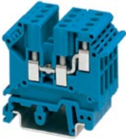
1-level terminal block with double connection on one side, cross section: 0.2 - 2.5 mm 2 , AWG: 30 - 12, width: 5.2 mm, color: blue
