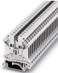
Feed-through terminal block, Connection method: Screw connection, Cross section: 0.2 mm 2 - 6 mm 2 , AWG: 24 - 10, Width: 6.2 mm, Color: white, Mounting type: NS 35/7,5, NS 35/15, NS 32
