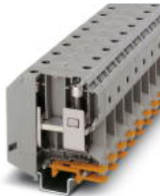
Feed-through terminal block, Connection method: Screw connection, Cross section: 25 mm 2 - 95 mm 2 , AWG: 4 - 3/0, Width: 25 mm, Height: 90 mm, Color: gray, Mounting type: NS 35/15, NS 32
