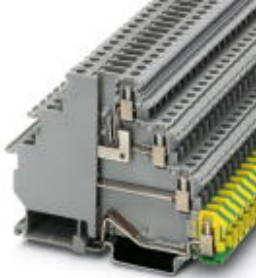
Sensor/actuator terminal block, Cross section: 0.2 mm 2 - 4 mm 2 , AWG: 24 - 12, Connection type: Screw connection, Width: 6.2 mm, Color: gray, Mounting type: NS 35/7,5, NS 35/15
