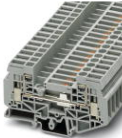
Slide-type terminal block, Connection method: Screw connection, Cross section: 0.5 mm 2 - 10 mm 2 , AWG: 20 - 10, Width: 8.2 mm, Mounting type: NS 35/7,5, NS 35/15, NS 32, Color: gray
