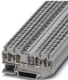
Component terminal block, Connection method: Spring-cage connection, Cross section: 0.08 mm 2 - 4 mm 2 , AWG: 28 - 12, Width: 5.2 mm, Color: black, Mounting type: NS 35/7,5, NS 35/15
