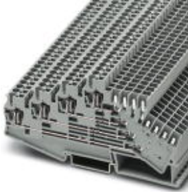
Multi-level terminal block, Connection method: Spring-cage/plug-in connection, Cross section: 0.08 mm 2 - 4 mm 2 , AWG: 28 - 12, Width: 5.2 mm, Color: gray, Mounting type: NS 35/7,5, NS 35/15
