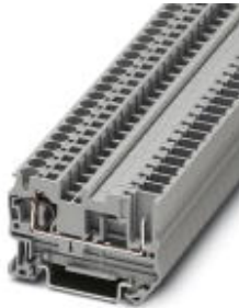
Feed-through terminal block, Connection method: Spring-cage/plug-in connection, Cross section: 0.08 mm² - 6 mm², AWG: 28 - 10, Width: 6.2 mm, Color: gray, Mounting type: NS 35/7,5, NS 35/15
