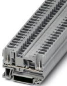
Feed-through terminal block, Connection method: Spring-cage/plug-in connection, Cross section: 0.08 mm 2 - 6 mm 2 , AWG: 28 - 10, Width: 6.2 mm, Color: gray, Mounting type: NS 35/7,5, NS 35/15
