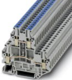
Feed-through terminal block, Cross section: 0.14 mm 2 - 6 mm 2 , AWG: 26 - 10, Connection type: Screw connection, Width: 6.2 mm, Color: gray, Mounting type: NS 35/7,5, NS 35/15
