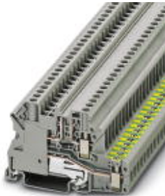
Component terminal block, Connection method: Screw connection, Cross section: 0.14 mm 2 - 6 mm 2 , AWG: 26 - 10, Width: 6.2 mm, Color: gray, Mounting type: NS 35/7,5, NS 35/15
