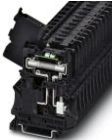
Lever-type fuse terminal block, black, for 6.3 x 32 mm G fuse inserts, with LED for 250 V AC
