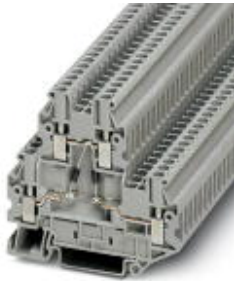
Component terminal block, Cross section: 0.14 mm 2 - 4 mm 2 , AWG: 26 - 12, Connection type: Screw connection, Width: 5.2 mm, Color: gray, Mounting type: NS 35/7,5, NS 35/15
