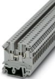
1-level terminal block with double connection on one side, cross section: 0.2 - 4 mm 2 , AWG: 24 - 12, width: 6.2 mm, color: White
