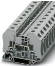
Feed-through terminal block with bolt connection, cross section: 0.1 - 2.5 mm 2 , AWG: 26 - 14, width 12.3 mm, color: Gray
