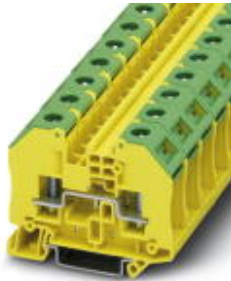
Ground terminal block with bolt connection, cross section: 0.1 - 6 mm 2 , AWG: 26 - 10, width 16.3 mm, color: Green-yellow
