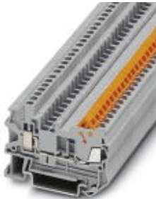
Feed-through terminal block, Connection type: Quick connection, Screw connection, Cross section: 0.25 mm² - 1.5 mm², AWG :24- 16, Width: 5.2 mm, Color: gray, Mounting: NS 35/7,5, NS 35/15
