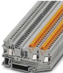
Feed-through terminal block, Connection type: Quick connection, Screw connection, Cross section: 0.25 mm² - 1.5 mm², AWG :24- 16, Width: 5.2 mm, Color: gray, Mounting: NS 35/7,5, NS 35/15
