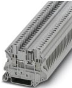
Component terminal block, Connection method: Screw connection, Cross section: 0.14 mm 2 - 4 mm 2 , AWG: 26 - 12, Width: 5.2 mm, Color: gray, Mounting type: NS 35/7,5, NS 35/15
