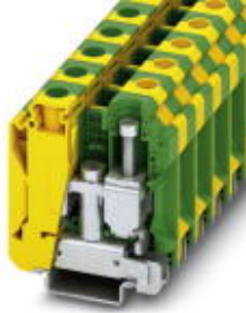
Ground modular terminal block, Connection method: Screw connection, Cross section: 10 mm 2 - 35 mm 2 , AWG: 8 - 2, Width: 16 mm, Color: green-yellow, Mounting type: NS 35/7,5, NS 35/15, NS 32
