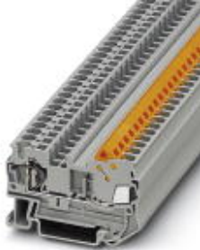
Feed-through terminal block, Connection type: Quick connection, Spring-cage connection, Cross section: 0.5 mm 2 - 2.5 mm 2 , AWG :20- 14, Width: 6.2 mm, Color: gray, Mounting: NS 35/7,5, NS 35/15
