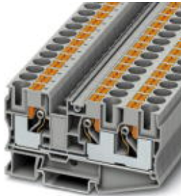
Feed-through terminal block, Connection method: Push-in connection, Cross section: 0.5 mm 2 - 16 mm 2 , AWG: 20 - 6, Width: 10.2 mm, Height: 49.5 mm, Color: gray, Mounting type: NS 35/7,5, NS 35/15
