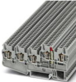
Sensor/actuator terminal block, Connection method: Spring-cage connection, Cross section: 0.08 mm 2 - 4 mm 2 , AWG: 28 - 12, Width: 5.2 mm, Color: gray, Mounting type: NS 35/7,5, NS 35/15
