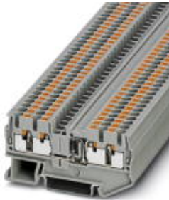
Component terminal block, Connection method: Push-in connection, Cross section: 0.14 mm 2 - 4 mm 2 , AWG: 26 - 12, Width: 5.2 mm, Color: gray, Mounting type: NS 35/7,5, NS 35/15
