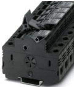
Fuse terminal block with light indicator, for cartridge fuse insert 10.3 x 38 mm, cross section: 1.5 - 25 mm 2 , AWG: 16 - 4, width: 18 mm, color: Black
