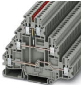
Component terminal block, Cross section: 0.14 mm 2 - 4 mm 2 , AWG: 26 - 12, Connection type: Screw connection, Width: 5.2 mm, Color: gray, Mounting type: NS 35/7,5, NS 35/15
